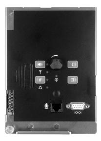
On power-up, the control panel selects Channel 1. During normal operation, pressing 'I' selects Channel 1 and pressing 'II' selects Channel 2. Pressing a channel select button when that particular channel has already been selected has no effect.
